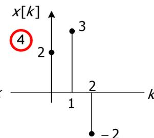
$$\begin{cases} n+1 < 0, & * = 0 \\ n+1 = 0, & * = 1 \times 2 = 2 \\ n+1 = 1, & * = 2 \times 2 + 1 \times 3 = 7 \\ n+1 = 2, & * = 1 \times 2 + 2 \times 3 - 2 \times 1 = 6 \\ n+1 = 3, & * = 1 \times 3 + 2 \times (-2) = -1 \\ n+1 = 4, & * = 1 \times (-2) = -2 \\ n+1 \geq 5, & * = 0 \end{cases}$$
