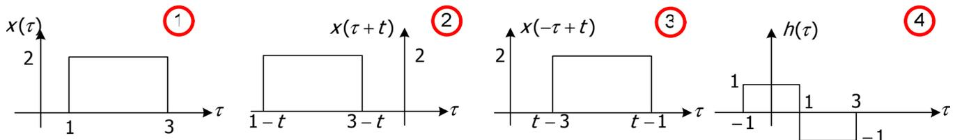
$$\left\{ \begin{array}{ll} t - 1 < 1 & , \quad * = 0 \\ -1 \leq t - 1 < 1 & , \quad * = \int_{-1}^{t-1} 2d\tau = 2t \\ 1 \leq t - 1 < 2 & , \quad * = \int_{t-3}^1 2d\tau + \int_1^{t-1} -2d\tau = 12 - 4t \\ 2 \leq t - 1 < 3 & , \quad * = \int_{t-3}^1 2d\tau + \int_1^{t-1} -2d\tau = 12 - 4t \\ 3 \leq t - 1 < 4 & , \quad * = \int_{t-3}^3 -2d\tau = -2(6 - t) \\ t - 1 \geq 5 & , \quad * = 0 \end{array} \right.$$
