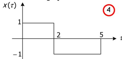
$$\left\{ \begin{array}{l} t-1 > 5, \quad * = 0 \\ 2 < t-1 \leq 5, \quad * = \int_{t-1}^5 e^{2(-\tau+t)} \times (-1) d\tau = \frac{1}{2} e^{2(t-5)} - e^2 \\ 0 < t-1 \leq 2, \quad * = \int_{t-1}^2 e^{2(-\tau+t)} d\tau + \int_2^5 e^{2(-\tau+t)} d\tau = \frac{1}{2} (e^2 - e^{2(t-2)} + e^{2(t-5)} - e^{2(t-2)}) \\ t-1 \leq 0, \quad * = \int_0^2 e^{2(-\tau+t)} d\tau + \int_2^5 -e^{2(-\tau+t)} d\tau = \frac{1}{2} (e^{2t} - e^{2(t-2)} + e^{2(t-5)} - e^{2(t-2)}) \end{array} \right.$$
