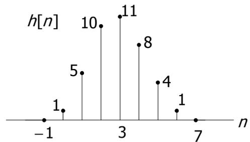
$$h_2[n] = \delta[n] + \delta[n-1] \quad , \quad h[n] = h_1[n] * (h_2[n] * h_2[n])$$
