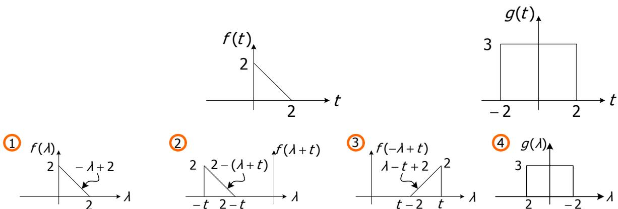
$$\left\{ \begin{array}{ll} t < -2 , & * = 0 \\ -2 \leq t < 0 , & * = \int_{-2}^t (\lambda - t + 2)(3) d\lambda = \frac{3}{4}(4 - t^2) \\ 0 \leq t < 2 , & * = \int_{t-2}^t (\lambda - t + 2)(3) d\lambda = 6 \\ 2 \leq t \leq 4 , & * = \int_{t-2}^2 (\lambda - t + 2)(3) d\lambda = \frac{3}{2}(t^2 - 8t + 16) \\ t \geq 4 , & * = 0 \end{array} \right.$$
